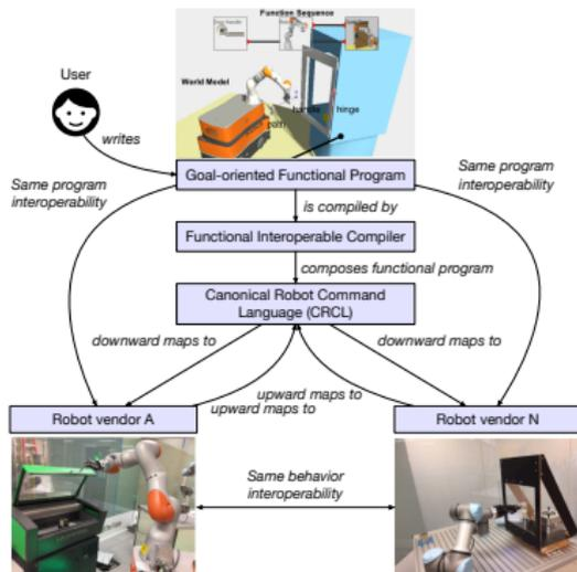
**Figure:** RoboCat framework consists of a goal-oriented functional programming environment, a functional interoperable compiler, and the mapping to the Canonical Robot Command Language (CRCL) and robot-specific APIs
